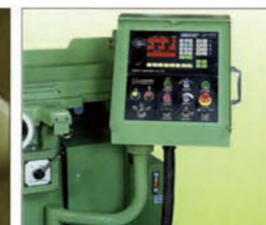
Control box with 2 revolving joints, position of the box can be adjusted easily for operation.
