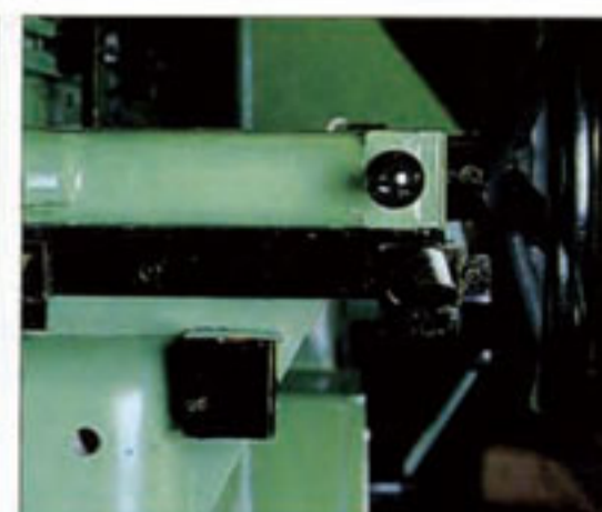
Non-contact proximity switches and dogs for cross feed stroke adjustment.
